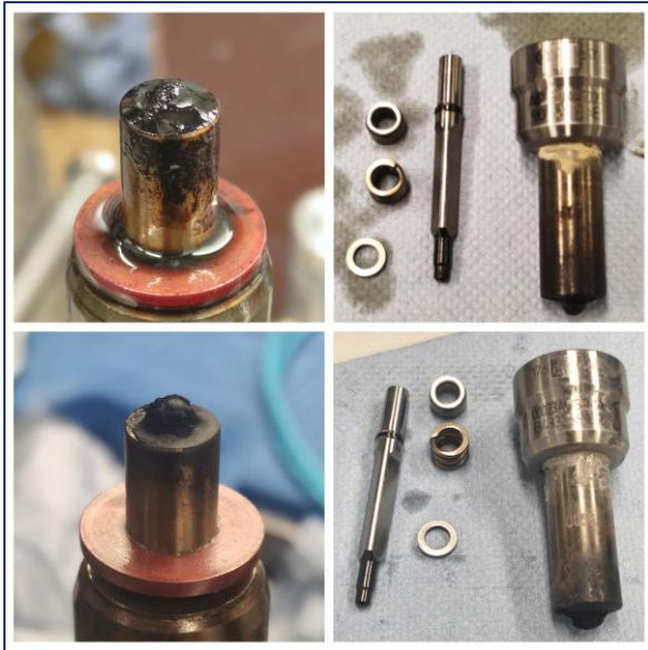
Figure 8: Injector nozzle directly after dismantling (left) and disassembled nozzle incl. needle (right); from the test runs with POCC B20 blend (upper) and unsuitable bio-blend (lower)
