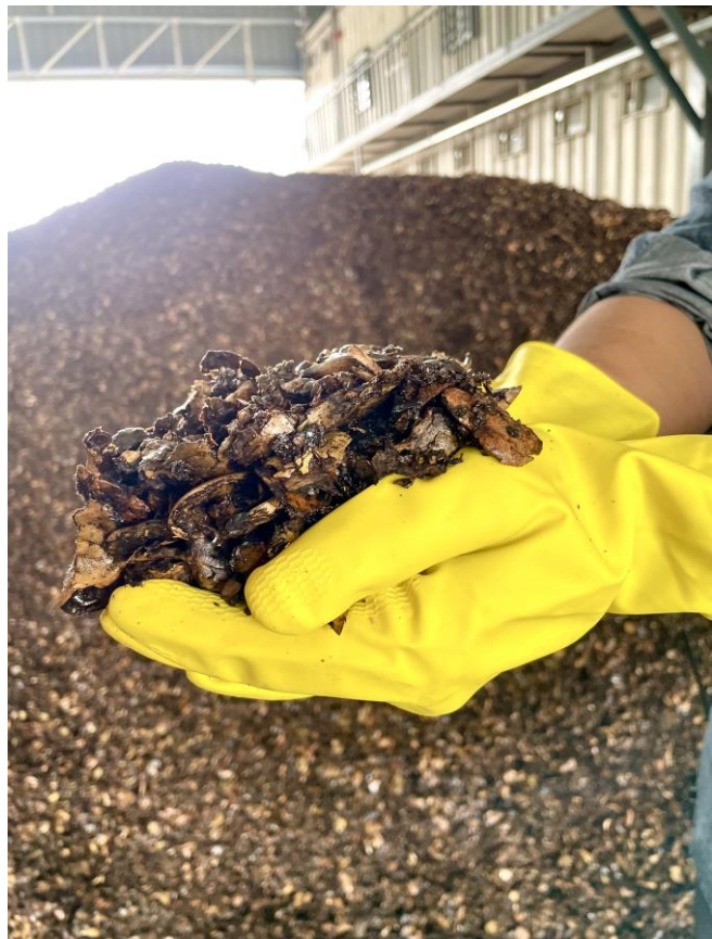
Figure 1: Cashew shell press cake before further pyrolysis treatment (source: MASH Makes)
