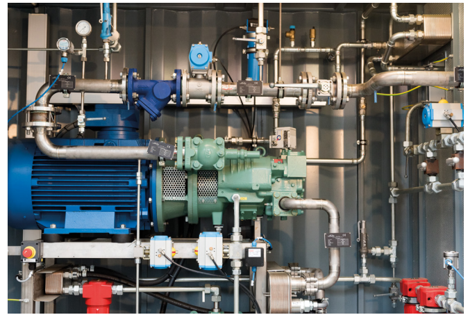
▲ 20 bar natural gas compressor
